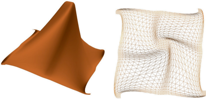
Figure III.4: The “Tower” surface: a blending spline tensor-product surface made up of 3 \times 3 knots with associated local plane surface patches. The local surfaces in the corners are locally rotated in the xy - and xz -planes. The rendering lattice, in this case, is made up of 3 \times 3 render loci (one for each spline knot locus) and four render patches. On the left is a shaded version of the resulting surface, while on the right is a wireframe version showing the tessellation of the four render patches.
